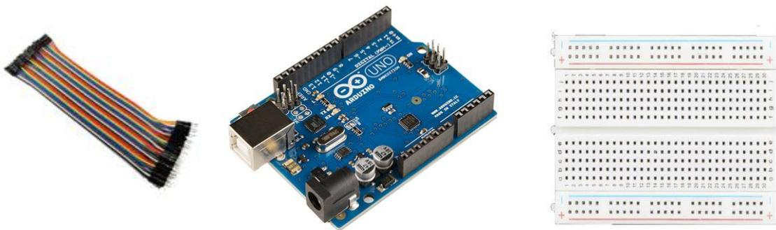
Figure 3-13: connecting wires, Arduino Uno chip, and breadboard
